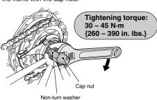
4. Fix the brake arm securely to the chainstay with the
