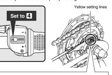
The yellow setting lines on the cassette joint are located in two places. Use the one that is easiest to
