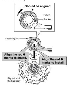
3. Secure the cassette joint to the hub with the cassette joint fixing ring. When installing the cassette joint fixing ring, align the yellow • mark with the yellow • mark on the cassette joint pulley, and then turn the cassette joint fixing ring 45° clockwise
