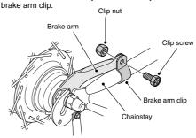
· When installing the brake arm clip, securely tighten the clip screw while holding the clip nut
