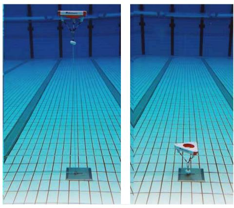
The ball release needs to have 2 underwater anchors + 1 deck anchor:
