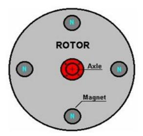
It needs to be remembered that the proportions of the magnets are for the magnet length to be more than the diameter, so in cases like this where circular magnet faces are to be used, the magnets will be cylindrical and the rotor needs to have a significant thickness, which will depend on the magnets which are available locally. The magnets should be a tight push-fit in their holes and securely glued in place.
