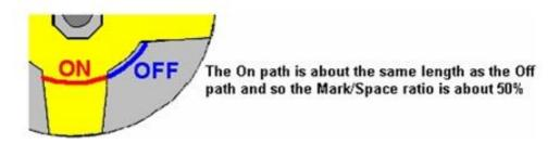
If, instead, the moveable brush is positioned near the outside edge of the disc, then because of the tapering of the copper arm, the On path is shorter and the non-conducting Off path is very much longer, being about three times as long as the On path, giving a Mark/Space ratio of about 25%. As the moveable brush can be positioned anywhere between these two extremes, the Mark/Space ratio can be set to any value from 25% to 50%.
