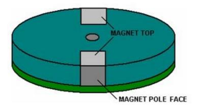
Here, the magnets are attached on the lower face, the right and left faces, and the unused pole face, and when the upper disc is attached, the upper faces are also secured and there is the minimum of air turbulence when the rotor spins:
