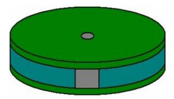
There is a "sweet spot" for the positioning of the power pick-up coils and it will usually be found that this is two or three millimeters away from the rotor. If that is the case, then there will be room for an outer band of duct tape on the rim of the rotor to provide additional protection against the failure of the magnet attachment method.
