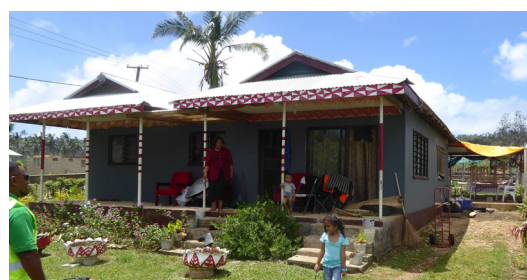
The roofs of these verandas are detached from the main roofs, reducing the risk of domino effect starting from them during storms. House in 'Eua. © Bill Flinn - Care
