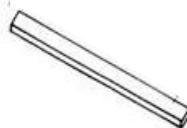
Leveling ruler to remove excess on the mould. If not available, it can be done by hand
