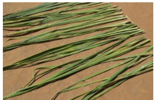
Sisal is also used for connections. Makhoma, Dowa. © Jon Twingi
