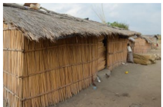
House built with timber or bamboo framework wattle and daub walls and thatched roof (thatch). © Jon Twingi
